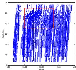
**Figure 2: Plot of individual trajectories produced by *GPS*; the red square indicates the space and time information of an accident. In the *Caltrans PeMS* website, the accident report recorded the accident for only one station (postmile 26.641); however, as shown in this plot, the accident propagates and gives effect to the upstream and (a little to) the downstream stations.**
