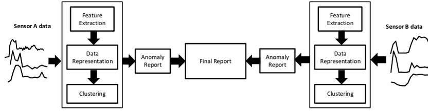
**Figure 3: The proposed anomaly detection method.** The final report is created based on the anomalies detected from different views, such as sensor readings of different locations, different types of sensors, different measurements, etc.
